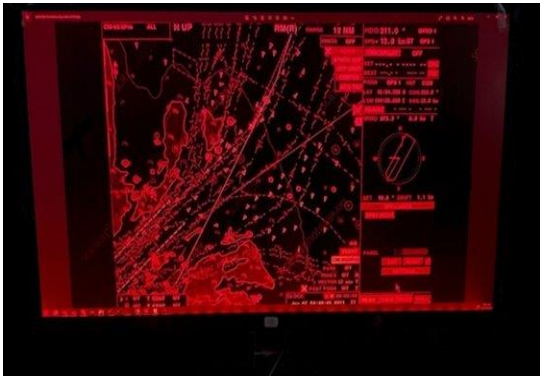
Red Mode selected which can be dimmed to support un-augmented night vision
