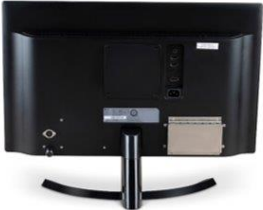
Back view of the Monitor with the driver module box installed on COTS monitors
