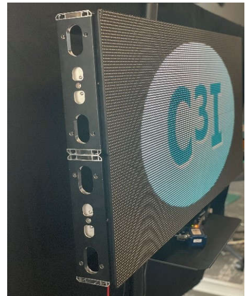
Side image of the extruded aluminum framework of the
